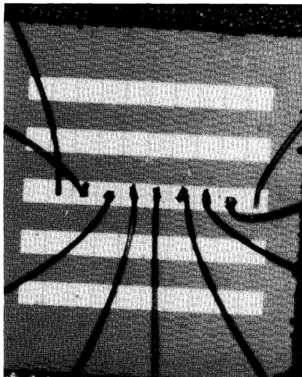
Fig. 2. First experimental array of field plates used to demonstrate the principles of charge transfer.
