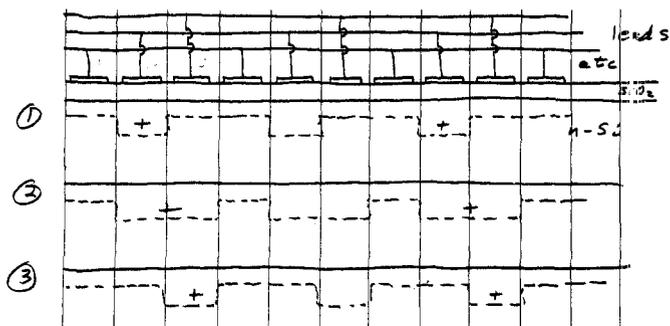
Fig. 1. Reproduction of the notebook sketch of the first three-phase charge-coupled device.
