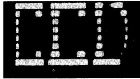
Fig. 4. Image produced by an 8-bit linear array of CCD elements. Scanning from left to right was obtained mechanically.
