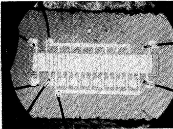
Fig. 3. The first 8-bit fully integrated device with diode inputs and outputs.
